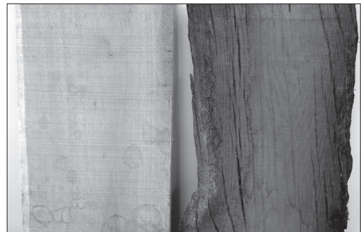
Figure 3. The colour difference and the large presence of cracks in subfossil oak wood (left), compared to recent oak wood (right)
