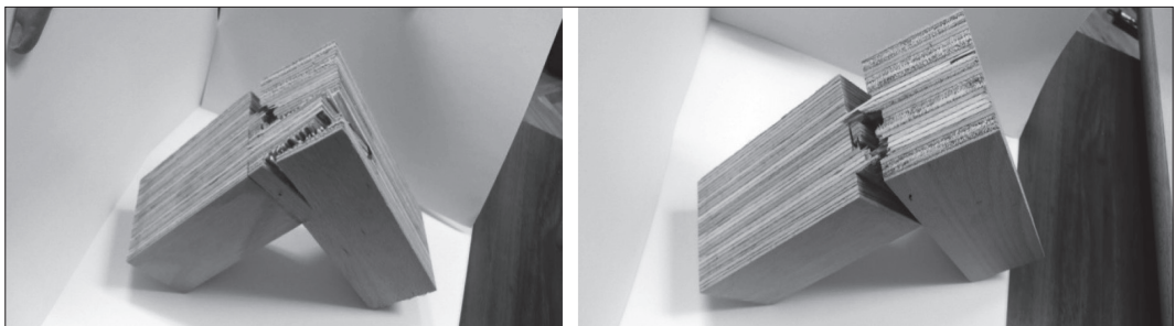
Figure 6. Left: Type „A“ failure, right: type „B“ failure
