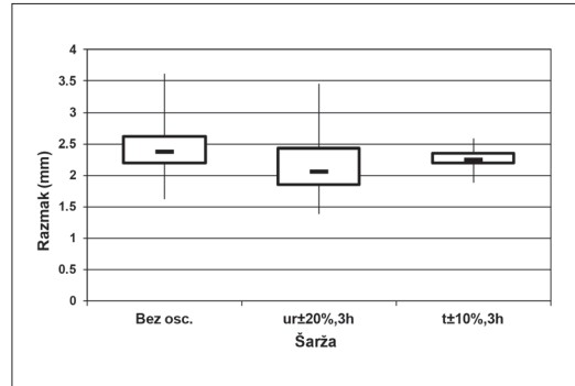
Figure 5. Values of gap after active drying phase (after 48 h of acclimatization)
