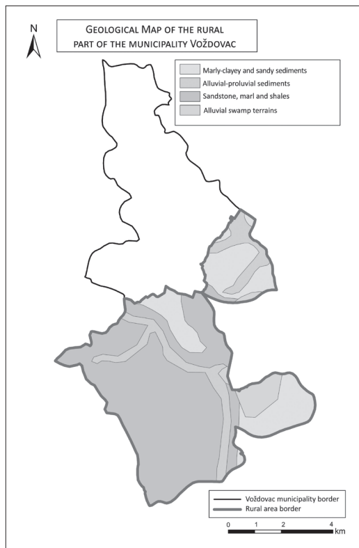
Figure 1. Geological map of the rural part of the municipality of Voždovac Source: Military Geographical Institute
