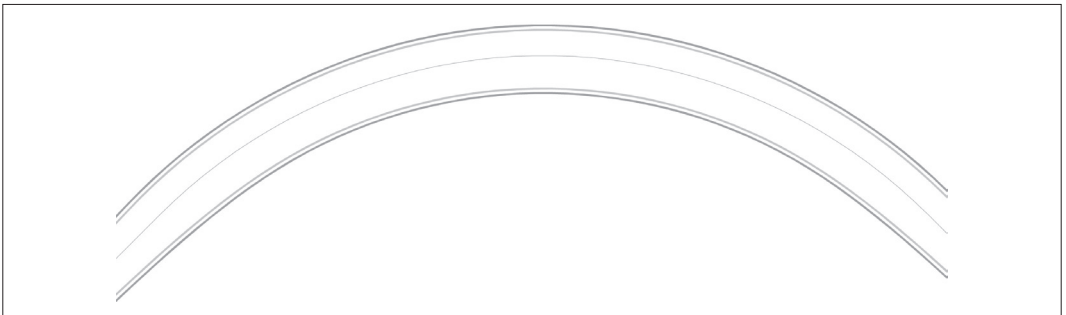
Figure 3d. Widening of a forest road traveled way edges for the width of a safety belt
