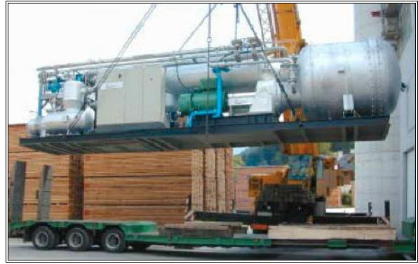
Figure 2 - The whole module of the biomass-fired CHP plant ([14])
