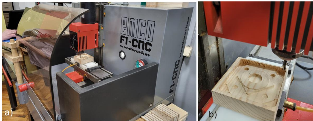
Fig. 12. Machined test workpiece with the vertical configuration of the machine
