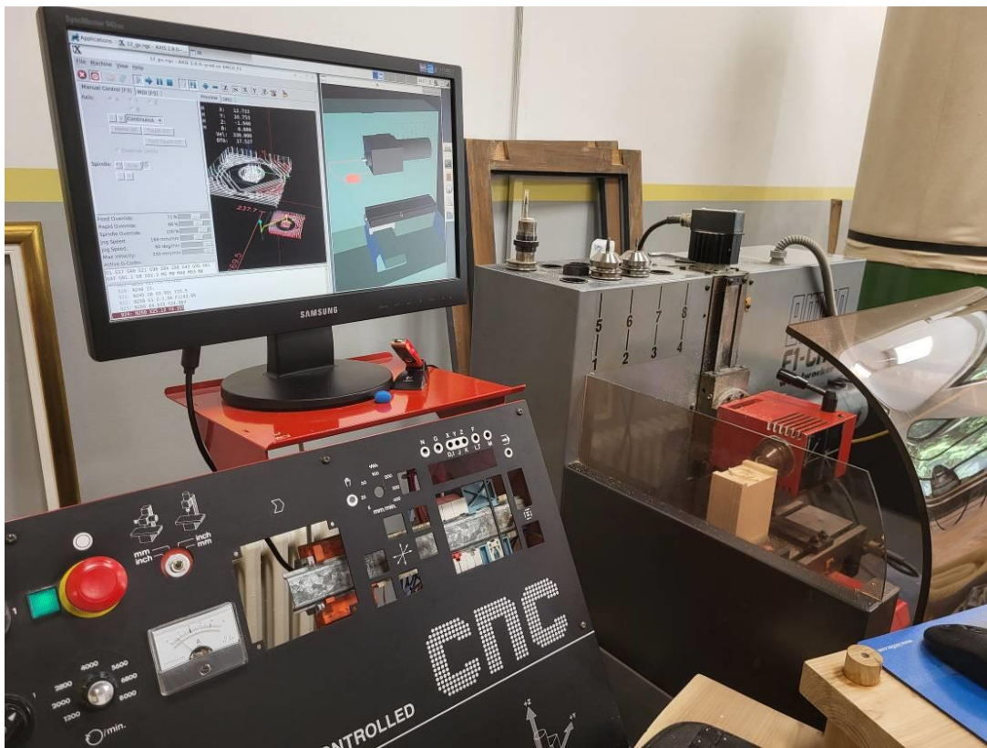
Fig. 11. Example of virtual woodworking CNC machine EMCO F1 integrated with a reconfigurable control system based on LinuxCNC
