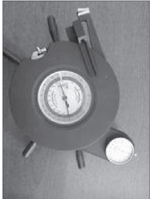
Figure 1. IML Fractometer 2 – a device for measuring the properties of the core samples
