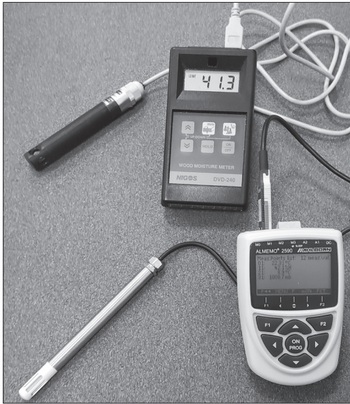
Figure 3. Capacitive probes for measuring temperature and relative humidity of the air
