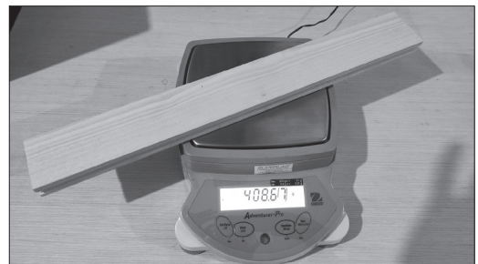
Figure 2. Mass measurement of the ash parquet element
