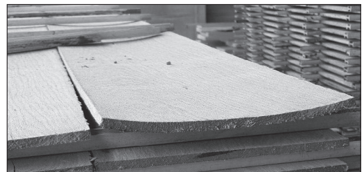
Figure 6. Cupping of a lamella from the highest row of the stack
