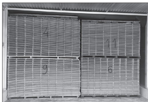
Figure 2. Stacked lamellas in the dehumidification kiln
