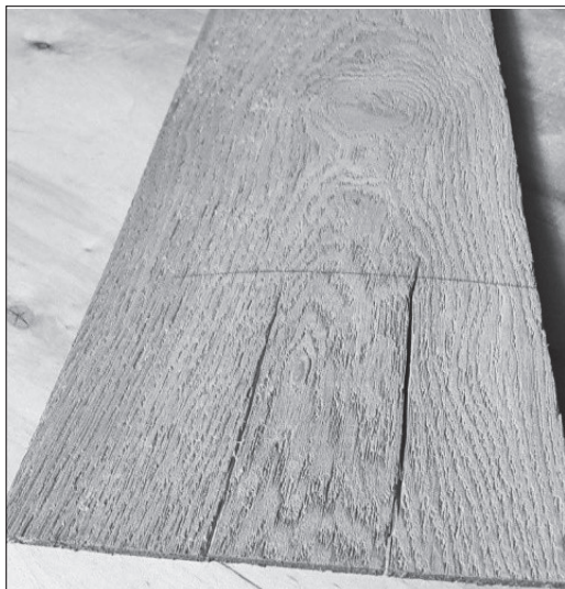
Figure 7. End checks on an oak lamella
